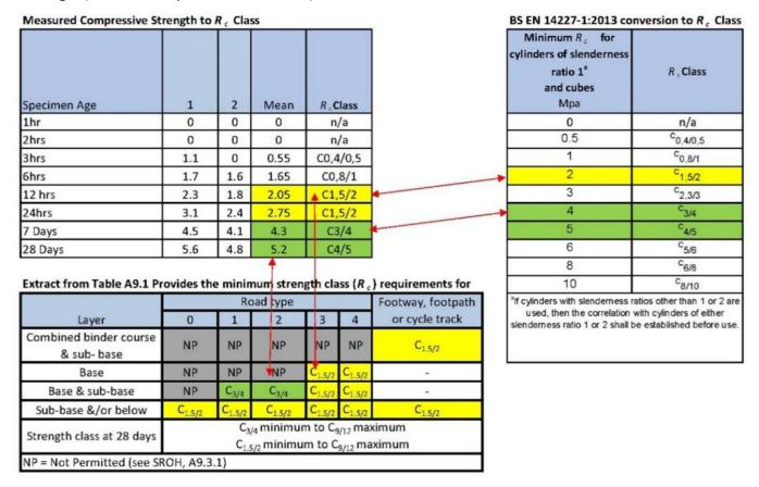
CBR data confirms Ultracrete Instafill/ Trenchfill exceeds the requirements for all classes of TMF (Treated Materials for Fills) materials within 4 hours of installation (CBR>15, Table 9.2, SROH)
